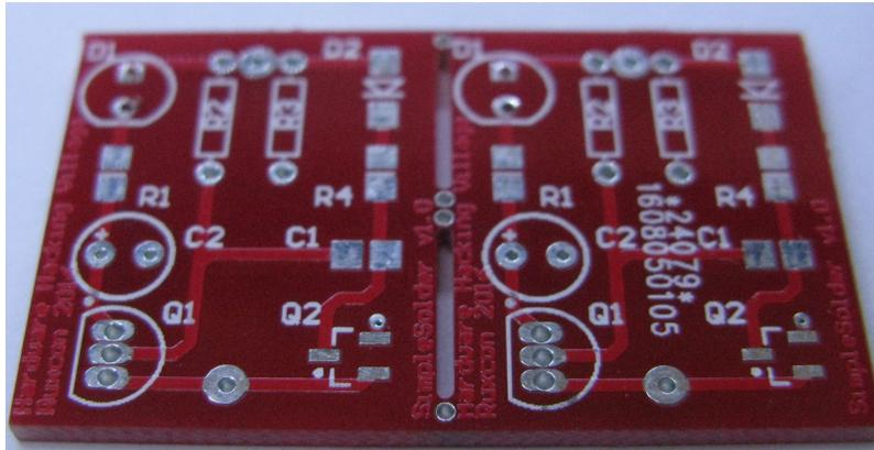
1. Each board is actually two boards. This guide only goes through populating the left hand board; the intention being that you can go and populate the right hand board yourself later (the boards can be snapped down the middle).
