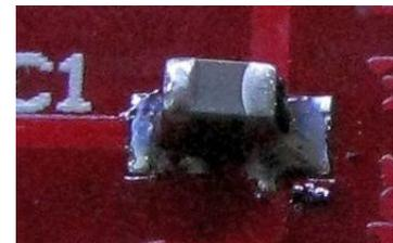
4. Repeat the process for the surface mount capacitor C1. Tin the pad, place the cap, hold it down while you touch the joint with your iron, then solder the other end.
