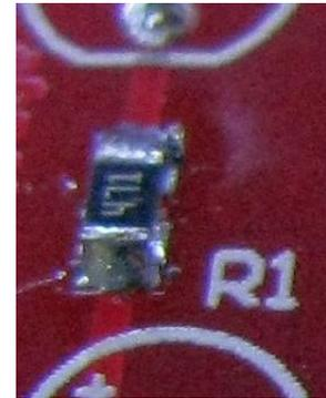
3. Next, place the resistors, positioning them so that one end is sitting on the tinned pad. Hold them in place with tweezers, then touch your soldering iron to the pad and the end of the resistor. The solder should flow onto the end of the resistor. Hold it in place for a moment while the solder freezes. After you've soldered the “tinned” end, apply solder to the other end of the resistor. Just a little dab will be enough; the end result should look similar to the above image.
