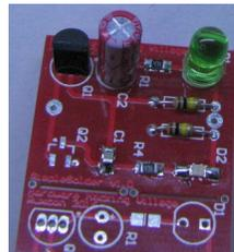
10. Next install the transistor. Note that the transistor should be installed **BACKWARDS** i.e. with the rounded side facing out.
