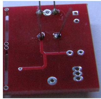
7. Grab two of your resistors and bend the leads at 90 degrees a few millimeters away from the body (left hand photo above), then insert them into the footprints on the board (R2 and R3). Once again, notice that they are installed such that they read (black brown yellow gold 100k 5%) the same way as the other components in this orientation on the board. Then flip the board over and solder the connections. Finally trim the leads off close to the board. Put one of your “pigtailed” aside.
