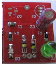
9. Next step is to install the through-hole capacitor (C2). Be careful with the orientation of this one too; the stripe on the can indicates the negative terminal, and it should be positioned in the orientation shown in the left hand photo (i.e. stripe facing “inwards”). Push it all the way down, flip the board over and solder both leads. Trim close to the board.
