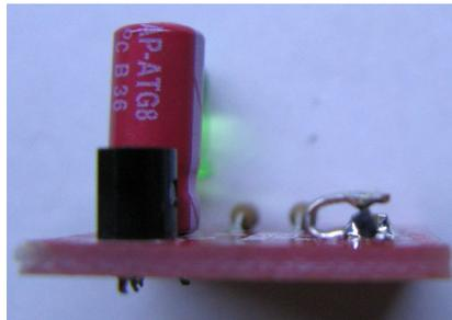
13. With your tweezers, position the transistor so that the two legs are sitting on the pads, then touch the pad you tinned with the soldering iron to flow the solder. Solder the other leg.
