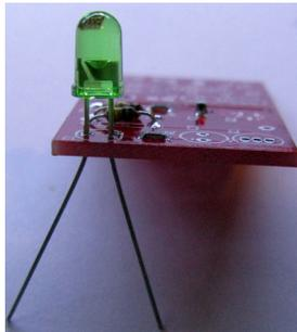
8. Next we're going to mount the through-hole LED. The holes in the design were too small for the leads of the LED so they had to be drilled out. This means that you will need to solder the LED on the TOP side of the board.
