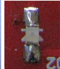
6. Make sure you orient the LED the right way around. If you look at the BACK of the LED you'll see a "T" shaped marking. That "T" shape corresponds to the highlighted "T" shape on the LED symbol next to it, which in turn corresponds with the marking on the PCB (this is the reverse of what it should be, it seems that Osram screwed up the markings on this batch of LEDs).
