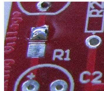
2. First we're going to solder the two surface mount resistors R1 and R4. The easiest way to do this manually is to "tin" one of the pads which basically entails applying a small amount of solder to the pad. (It's easiest to use fine solder for surface mount and thicker solder for through-hole parts) In the above image the topmost pads of R1 and R4 have been "tinned".
