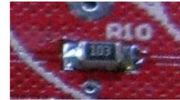
5. Now we move onto the top of the board. First we'll mount the 10k Resistor R10. Notice the marking 103, and also the fact that the resistor is "dressed" such that it reads correctly with when the board markings are the right way around.
